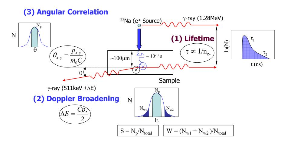
Positron Annihilation Spectroscopy consists of three techniques viz., (1) Positron lifetime (2) Doppler Broadening and (3) Angular Correlation of annihilation radiation.
